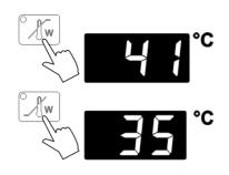
Display and adjustment of over-/undertemperature:
